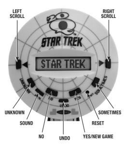
PORTABLE PLAY - To detach 20QTM STAR TREK from the stand, pull the hull up and off the stand. To separate the disc portion from the hull, pull the hull down and away from the disc portion. To reattach the disc and hull, press disc firmly into the corresponding pegs at the tip of the hull.
